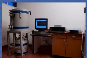
High Precision cooled HpGe Gamma Spectrometer
