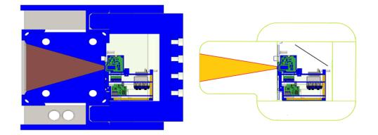
Figure 1 Side view of existing collimator (left). The blue regions represent tungsten. On the right is a concept for a smaller collimator that includes reducing the collimator opening angle and the internal volume for the electronics.
