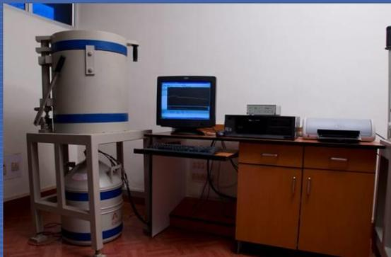
High Precision cooled HpGe Gamma Spectrometer
